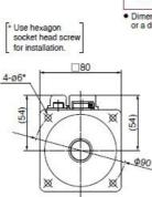
Motor model Mass: 1.5 kg Power supply Shaft Motor model No. MQMF041L1A1 Round 100 V MQMF041L1S1 Key-way, center tap MQMF042L1A1 Round 200 V Key-way, center tap MQMF042L1S1
